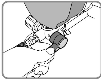
13. Turn Spray/Prime Switch to Spray mode and continue to spray into waste bucket.
