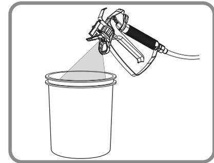
12. Switch power ON. Point gun into waste bucket and pull trigger.
