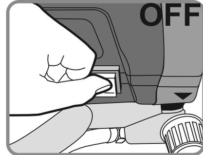
13. Release trigger, turn power OFF and turn Prime/ Spray switch to Prime mode to relieve pressure.
