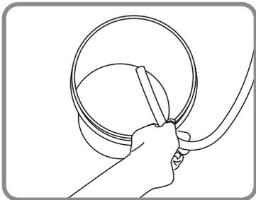
10. Paint should work itself from Suction Tube to Sprayer to Priming Tube until paint discharges from Priming Tube.
