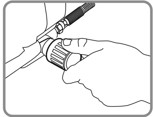
3. Turn Pressure Control Knob to Low Pressure Spray setting.
