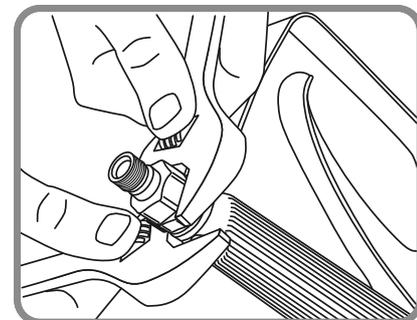
14. Unscrew nut from housing, it is **behind** the swivel connector.
