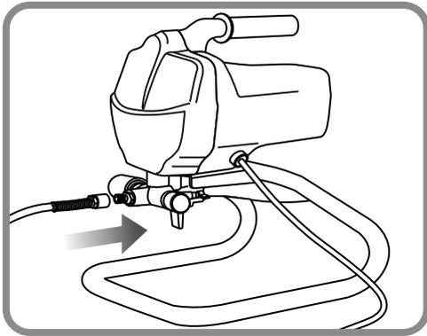
1. Attach Paint Hose to Paint Hose Outlet and tighten with wrench.
