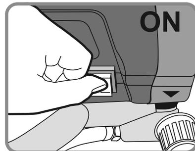
6. Plug in Sprayer and turn power ON.
