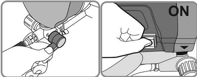
8. Turn to Spray mode and switch power to ON.
