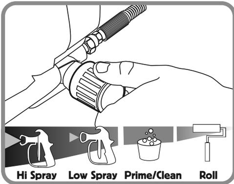
2. Start spraying at the lowest setting on the Pressure Control Knob and increase pressure as needed by turning clockwise to create a good spray pattern.
