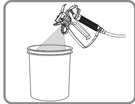
3. Point gun into paint pail and activate Sprayer Trigger to relieve any remaining pressure.
