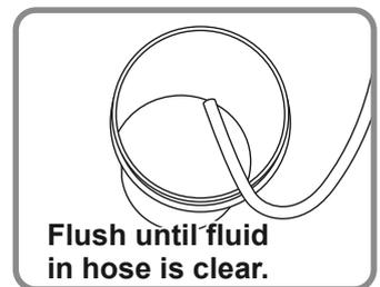
6. Plug in Sprayer and turn power ON. Sprayer will start pumping and water or flushing solvent as well as air bubbles will be purged from system. Let fluids discharge from Priming Tube into waste bucket until fluid is clear.
