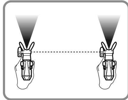
3. Keep gun straight and move arm across at a steady rate while staying one foot from the surface.
