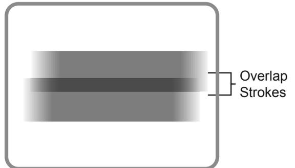
5. Overlap strokes by half. Always aim stroke at bottom edge of last stroke.
