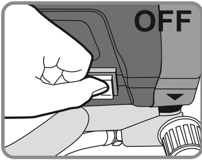
7. After fluid in Priming Tube is clear, switch Power to OFF.
