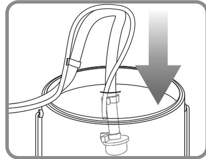
11. Switch power OFF. Remove the Priming Tube from the waste bucket and clip to Suction Tube and submerge in paint pail.
