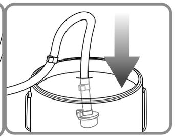
4. Place Priming Tube in empty waste bucket and submerge Suction Tube in water or flushing fluid.
