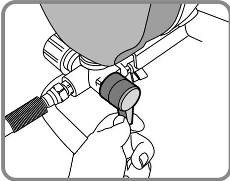
2. Switch Prime/Spray switch to Prime mode to safely release most pressure.
