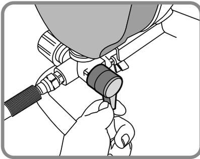
1. Turn power OFF and turn Prime/Spray switch to Prime mode to relieve pressure.
