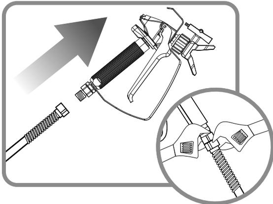
2. Attach Paint Hose to Paint Gun and tighten with two wrenches.
