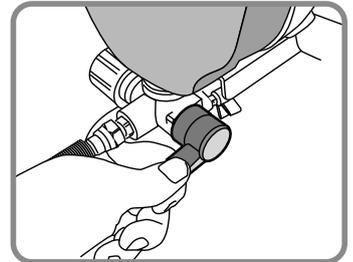
2. Turn the unit over and loosen the Clamps from both Tubes, then disconnect Tubes from the Pump Body.
